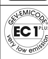
EMICODE: Classification system (GEV) of emission properties for construction products in indoor areas. EC-1 Plus (Very low emission Plus)
